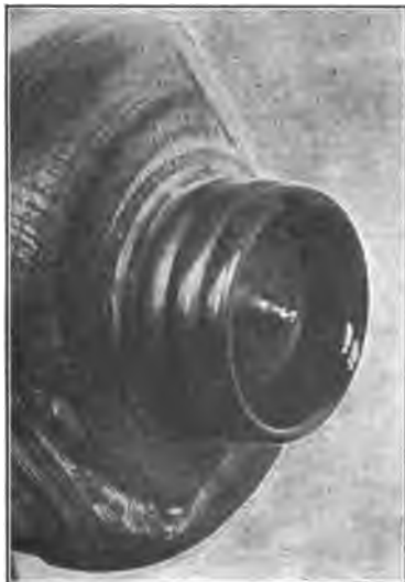
Fig. 167. Ring Turned on Screw Chuck.
